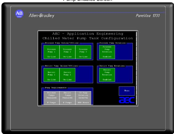
Any pump that is disabled to the OFF-LINE position will not be called to operate. Simply press the button of the desired pump to
